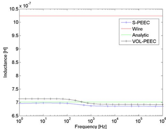
Fig. 1. Inductance of the rectangular bar obtained by means analytical formula (green), PEEC surface formulation (blue), and PEEC volumetric formulation (black). The inductance of a cylinder having the same dc resistance is also shown (red).
