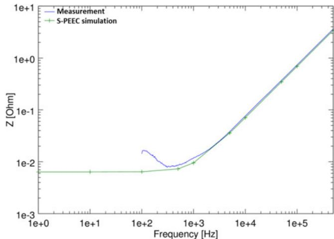
Fig. 8. Measured and simulated impedance of the test sample made by the cable over the U bar.
