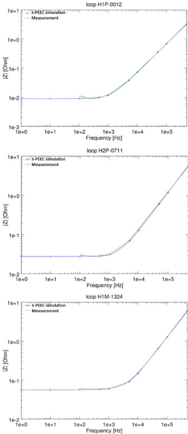
Fig. 10. Simulated and measured impedance (module) for three loops in different harnesses.
