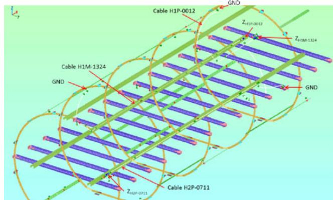
Fig. 9. Path of the three loops considered in Fig. 10. Cables are shown in white. GND indicates the connection point to the ALEEN structure. Z indicates the two terminals where the impedance is measured. The nose and the fuselage are not shown for clarity.
