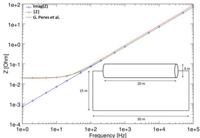
Fig. 6. Reactance (blue) and impedance (green) of the large cylinder shown in the inset. Data from [28] are also included (red).
