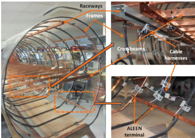
Fig. 3. Elements of the mock-up.
