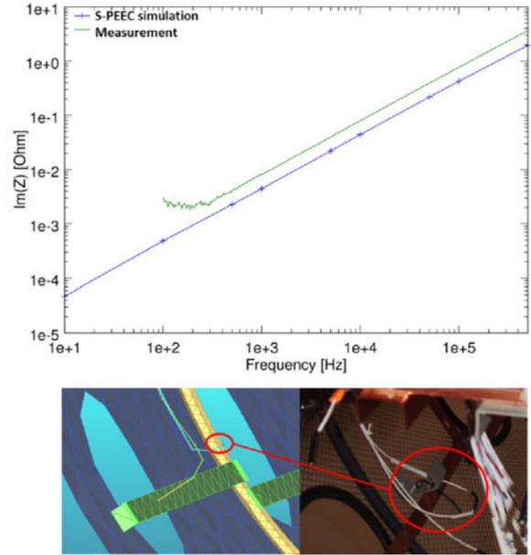
Fig. 11. Imaginary part of the impedance for a case with significant difference between measured (green) and simulated (blue) data. The difference is due to a loop not present in the numerical model (bottom).
