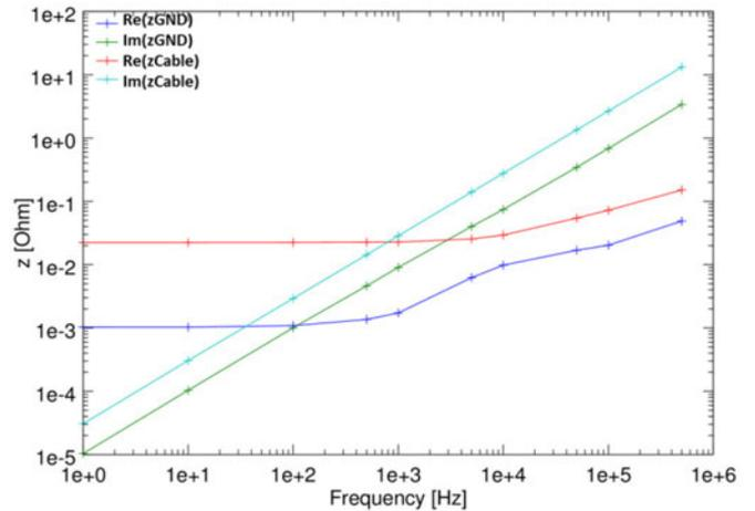
Fig. 12. Resistance and reactance of a cable and of ALEEN between the ground terminals of the cable itself.
