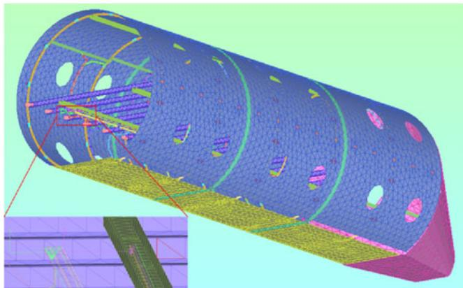
Fig. 4. Image of the numerical mock-up (mesh). The inset shows a particular of one side of two harnesses.
