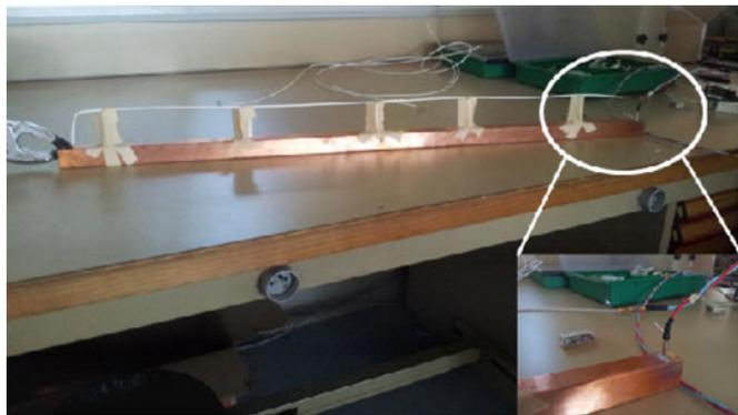
Fig. 7. Test sample used in validation. The 12 AWG cable is placed 5 cm over a copper U bar. The inset shows the two terminals of the loop.
